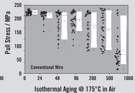
Bonding Condition: Metallization: 0.5% Cu, 99.5% Al · Bond pad pitch: 35 μm · Bonded ball diameter: 28 μm Wire diameter: 15 μm
