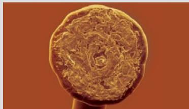
The SEM photographs above show evidence that the intermetallic penetration of the copper ball bond (above left) is significantly less than in the gold ball bond (above right). While this may raise questions as to the integrity of the bond, mid-span pull force tests show an average value of 44.6 grams (3.2 gr Sigma) and shear strength values of 6.5 gr/mil<sup>2</sup>; values that are, at least, comparable to those obtained with gold wire.
