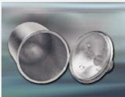
Boiling chamber according to DIN 52 322, diam. 40 cm
